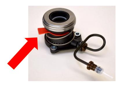
Failure to do so will cause damage to the CSC when the transmission is installed
