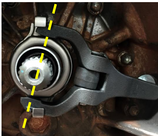
Image 1) Incorrect Fork Location
