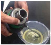
Step 3. Slowly compress the bearing down releasing the air inside of the slave cylinder until the bearing is fully compressed. Make sure that the inlet hose stays fully submerged during this process.
