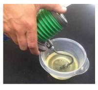
Step 4. Slowly release the bearing back up allowing the fluid to be drawn into the hydraulic cylinder. Make sure that the inlet hose stays full submerged during this process.
