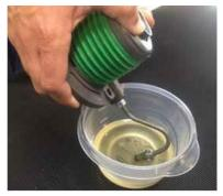
Step 2. Submerge the inlet hose of the slave cylinder into the brake fluid ensuring that the line cannot intake any air
