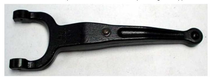
Make sure not to over stroke the release mechanism travel required to disengage the clutch as this may cause disengagement issues as the diaphragm spring or bearing comes into contact with the clutch disc hub.
