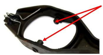
The forks in these vehicles are fitted with rubber absorbers at the contact points with the bearing.
