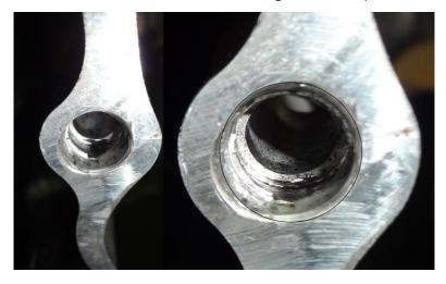
If misalignment has occurred it is recommended that the dowels are replaced and damage to the locating holes cleaned up as best as possible.
