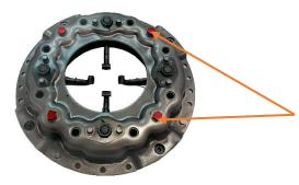
Hold Down Bolts need to be removed AFTER clutch is mounted to the flywheel and BEFORE installing gearbox. These are commonly painted red, If not, they will be located between the release leavers as per image.
