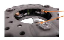
Blocks between the cover and the levers need to be removed AFTER clutch is mounted to the flywheel and BEFORE installing gearbox
