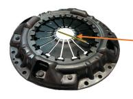
Wire Spacer Ring located between the cover and diaphragm needs to be removed AFTER clutch is mounted to the flywheel and BEFORE installing gearbox.
