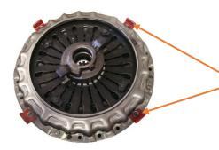
Red painted Hold Down Plates need to be removed AFTER clutch is mounted to the flywheel and BEFORE installing gearbox.
